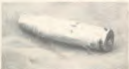
Fluted chamber shortens life of case. Violent extraction also damages cases. Later problem can be eliminated by removing ejection port flange.
